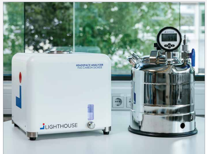
Figure 1: CCI test vessel and carbon dioxide headspace analyzer, used in the study described in this article.
