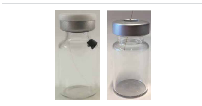
Figure 2: Left) Example of a positive control where a microwire is placed between the vial neck and the stopper. Right) Example of a positive control where a microcapillary is placed into a rubber stopper.
