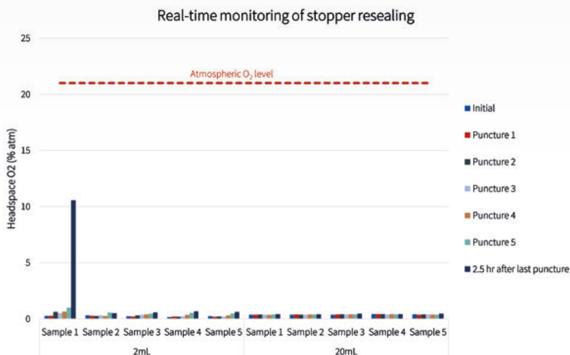
Figure 2 — 2mL and 20mL vials were stoppered and sealed under a nitrogen atmosphere. The vials were then punctured multiple times, and headspace oxygen measurements were made directly after each puncture.
